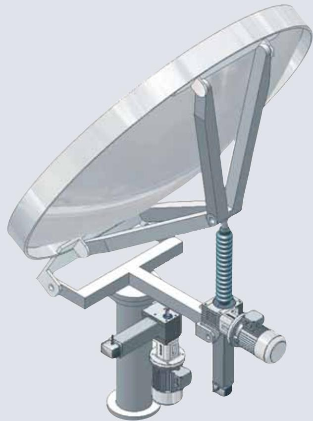
Parabolic Antenna  $\varnothing = 3,3$  m
