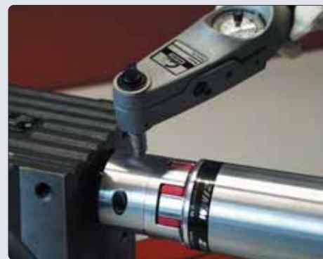
*Set screw tightening torque acc. to table*
